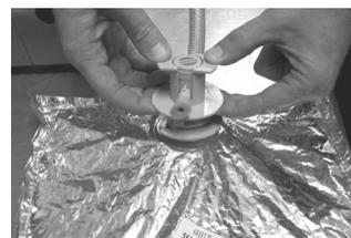
6. Push QCD plunger into bag spout until plunger top is flush with top of QCD. A “click” will be heard when it is fully inserted.
