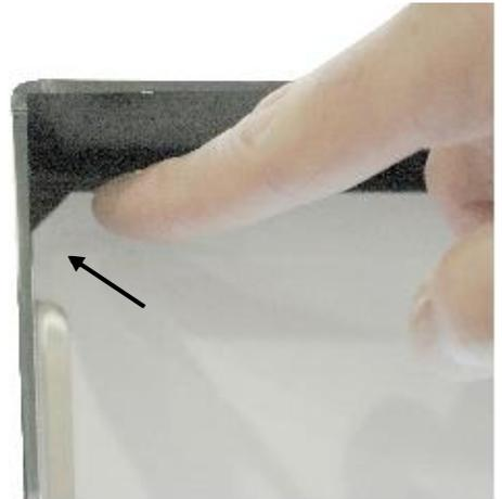
4. Gently remove one side by slightly bending the transparency to release from sliders.
