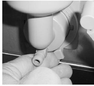
3. Rotate tab at bottom of mixing chamber bases counter clock wise to release base.
