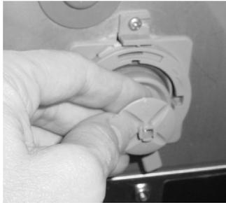
5. Remove frother disk from shaft by pulling straight out.
