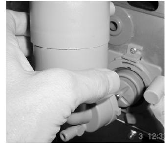
4. Remove mixing chamber and steam collector by pulling straight out.
