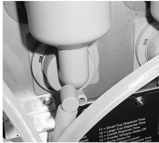
2. Remove elbows from mixing chambers, twisting slightly to help release.
