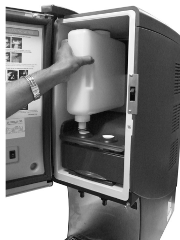
Figure 5. Loading a Concentrate Container
