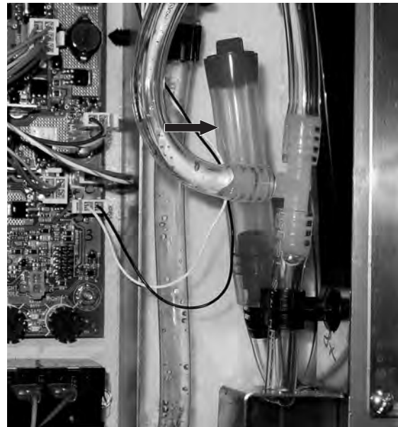
FIG 4 Initial Fill Hose - JDF-4S
