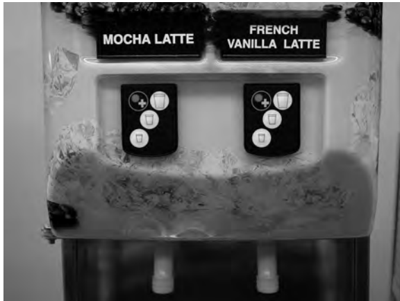
FIG 11 Product Dispense Switches - JDF-2S
