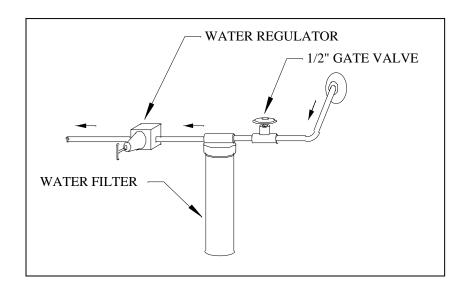
FIGURE 2-4. SUGGESTED WATER FLOW INSTALLATION
