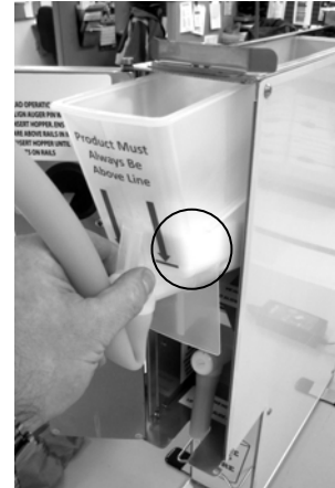
Side of hopper showing locking tab
